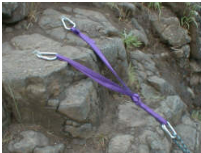
Figure 3: top rope anchor using 4 carabiners and a double length sling knotted at the focal point If the direction of the pull cannot be estimated accurately or when wide swings of the
